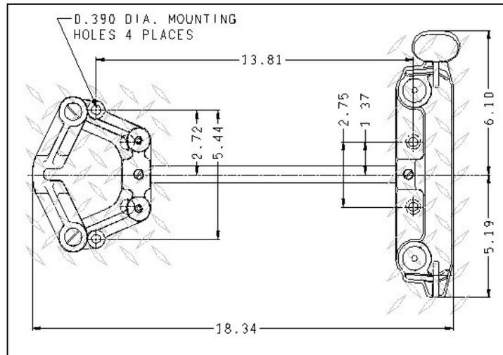
This bracket is designed to store the complete Stinger® portable monitor assembly upper unit (including nozzle and stream shaper) attached to portable base (all inlet configurations), or it can be used to store the portable base only.
