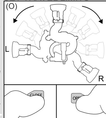
Lower Left: Move to top/right corner of the lower left zone, hold <Preset>, press <Close>, and release both.
