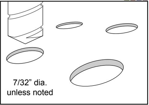
B. Drill holes for CAN network and power cables for each components' leads behind each component.
