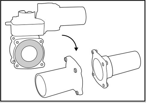
Tighten Adapter Bolts using a cross pattern
