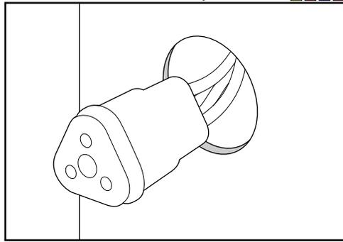
C. Mount components to panel using 10-24 x 1/2" screws. Use Loctite 242 or equivalent.
