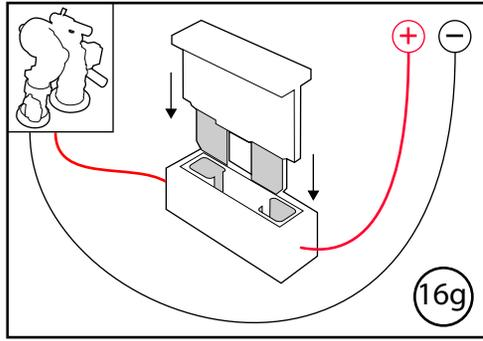
NOTE: We recommend using 14 AWG for monitor power and ground (12 AWG if using nozzle with foam expansion tube). See installation instructions section of the Scorpion EXM manual (98342000) for length to gauge recommendations.
