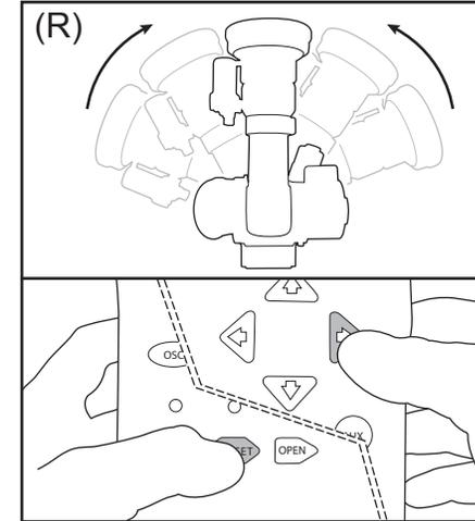
Aim monitor at center forward "zero" position. Hold PRESET, then press and release LEFT or RIGHT. The Status LED on monitor should blink and return to solid. Release PRESET button.
