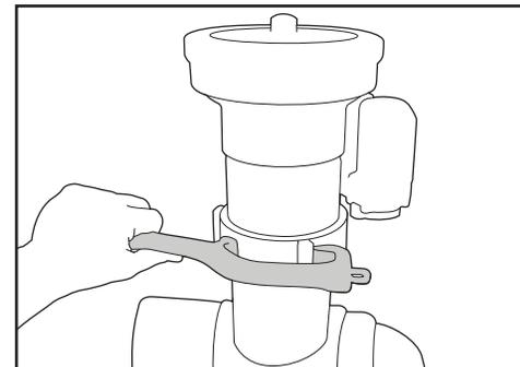
Tighten swivel using a spanner wrench to ensure a secure connection.
