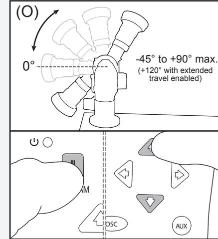
Upper: Move monitor to highest point of travel. Hold STREAM, then press UP, and release both.
