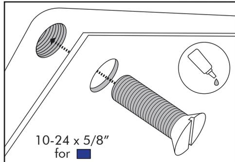
Mount components using 10-24 x 1/2" screws. Use Loctite 242 or equivalent.
