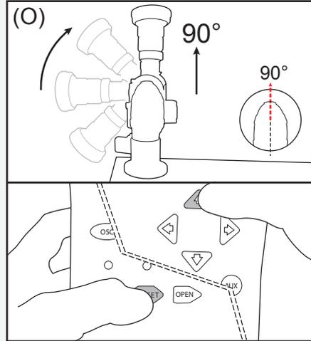
Aim monitor at the uppermost limit of travel. Hold PRESET, then press and release UP. The Status LED on monitor should blink and return to solid. Release PRESET button.
