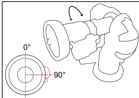
Hand tighten nozzle to monitor using swivel. Position actuator assembly about 90° as shown above.
