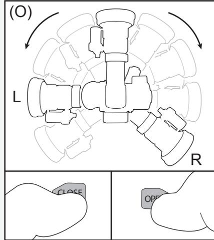
Move monitor to the left limit and press CLOSE. Move monitor to the right limit and press OPEN.
