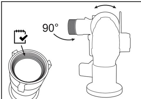
Position monitor discharge elbow parallel to the ground. Ensure gasket is inside nozzle swivel before installing.
