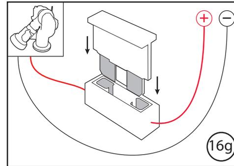
Install a 20A fuse (12VDC) into the positive power lead; 10A fuse for 24VDC.
