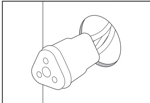
Drill holes for CAN network and power cables for each component.
