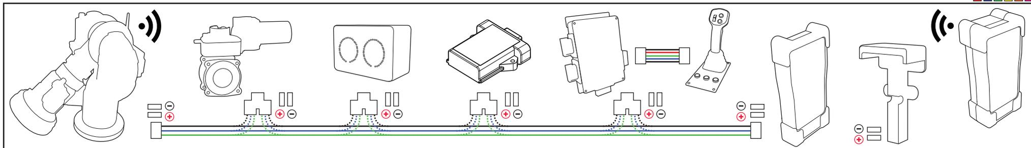
Connect entire CAN network together using 18-20 AWG. Ensure every component connected to the CAN network is connected in between the two (2) end components that have CAN termination. Please refer to the BLUE, GREEN, and BLACK lines as the CAN wires below.
