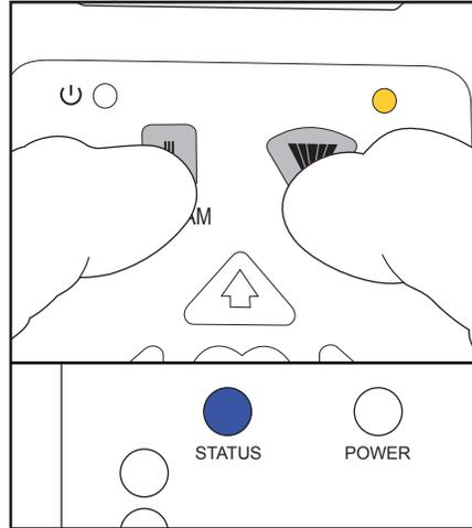
On the Handheld, press and hold FOG & STREAM buttons for 5 sec. (AUX & PRESET on Joystick). Blue Status LED on monitor & yellow LED on controller will be lit.
