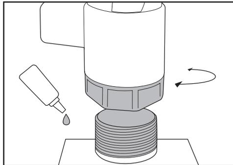
Thread monitor onto base using Loctite 592 thread sealant or equivalent. Tighten using strap wrench on hex portion of monitor base.
