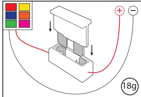
Install a 1A fuse (12VDC) into the positive power lead; 0.5A fuse for 24VDC.
