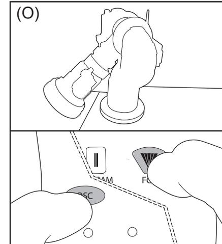
Move monitor to desired position, then press FOG and OSC at the same time to store a stow position.
