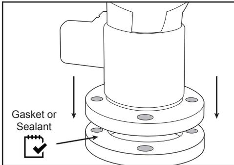
Install monitor to flange using 5/8"-11 UNC Grade 5 bolts and nuts. Tighten uniformly (20 lb increments) to 60-70ft/lb using Loctite 242 or equivalent.
